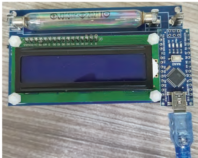
Figure 1. The Geiger-Müller counter kit (CAJOE, Model: GC-1602-NANO) is equipped with a J305 \beta\gamma Geiger tube and an arduino nano circuit board. This experiment did not use the LCD screen shown in the figure.
