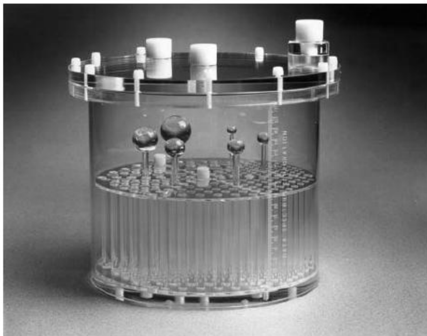
FIGURE 1. Jaszczak Deluxe Flangeless ECT Phantom.
