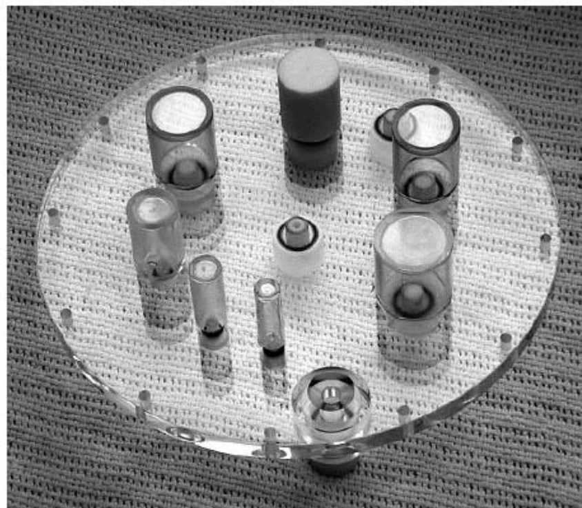
FIGURE 2. Modified faceplate used with Jaszczak Deluxe Flangeless ECT Phantom for PET phantom acquisition.
